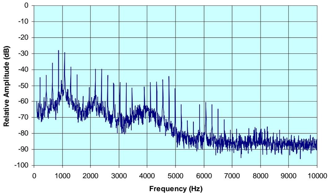
**Figure 5: Spectral response of interference produced in a radiofrequency low immunity hearing aid at maximum volume control and placed 1 metre from a 1750MHz GSM Mobile transmitting on full power.**
