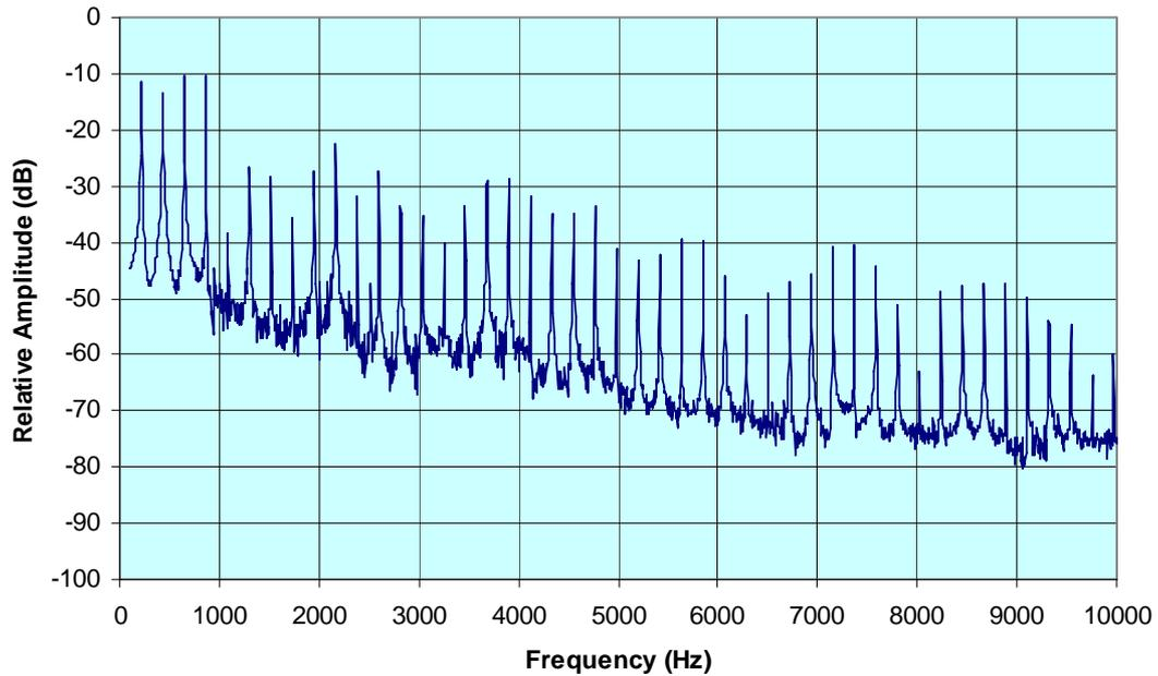
**Figure 4: Spectral response of interference produced in a radiofrequency low immunity hearing aid at maximum volume control and placed next to a 1750MHz GSM Mobile transmitting on full power.**
