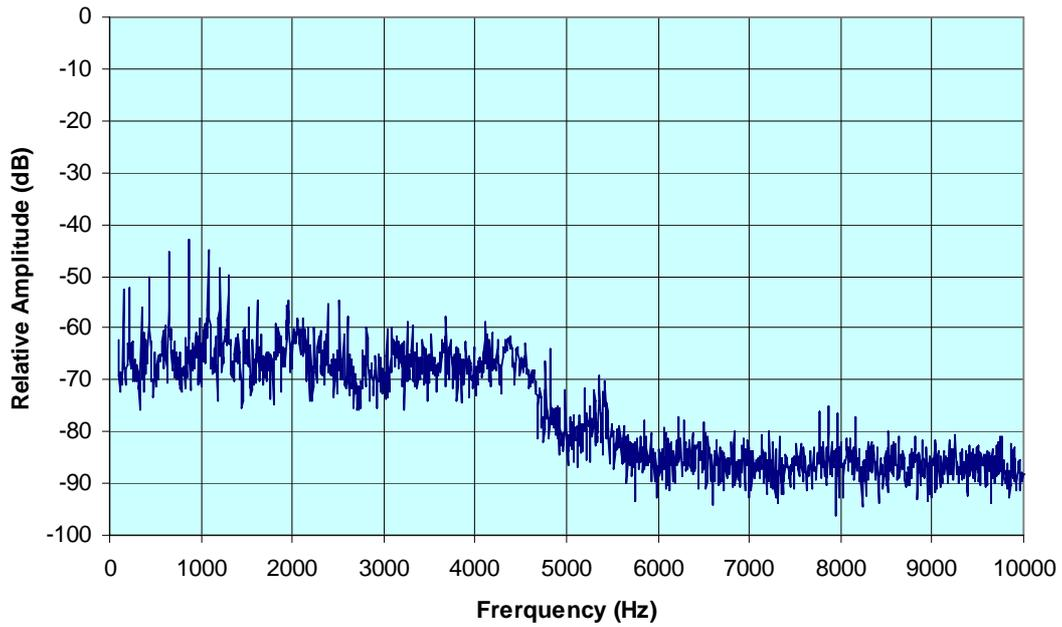
**Figure 8:** Spectral response of interference produced in a radiofrequency medium immunity hearing aid at reset volume control and placed next to a 1750MHz GSM Mobile transmitting on reduced power, -13.4 dB re maximum output (nominally -14 dB re maximum output).
