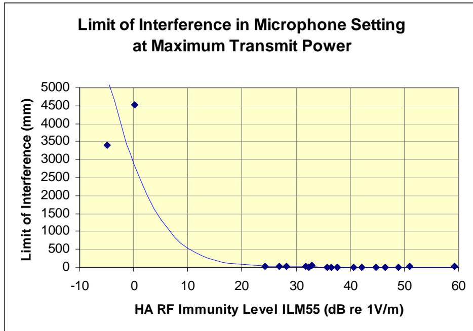
Figure 15: The limit of interference for the hearing aids used in the final study when in microphone setting.
