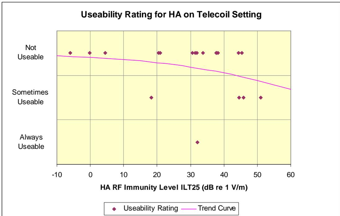
**Figure 20: Useability rating of interference produced in hearing aids in telecoil setting by a 1750 MHz GSM mobile telephone operating at maximum transmit power level and held in normal listening position.**
