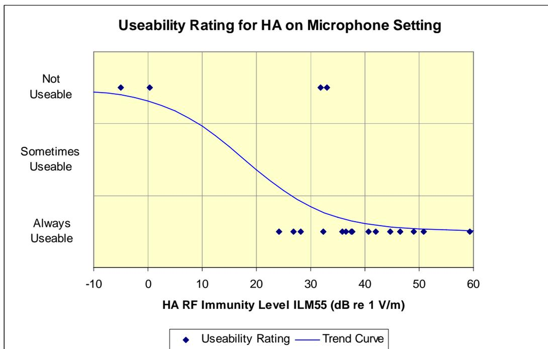
**Figure 18: Useability rating of interference produced in hearing aids in microphone setting by a 1750 MHz GSM mobile telephone operating at maximum transmit power level and held in normal listening position.**
