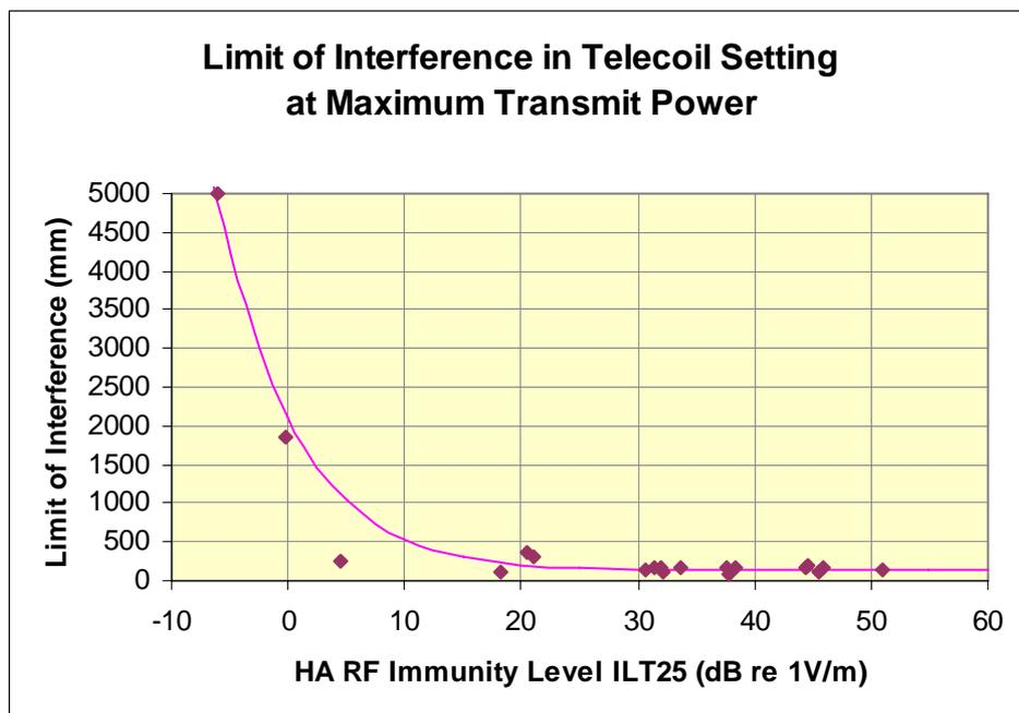
Figure 16: The limit of interference for the hearing aids used in the final study when in telecoil setting.
