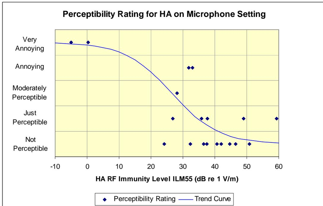
**Figure 17: Perceptibility rating of interference produced in hearing aids in microphone setting by a 1750 MHz GSM mobile telephone operating at maximum transmit power level and held in normal listening position.**
