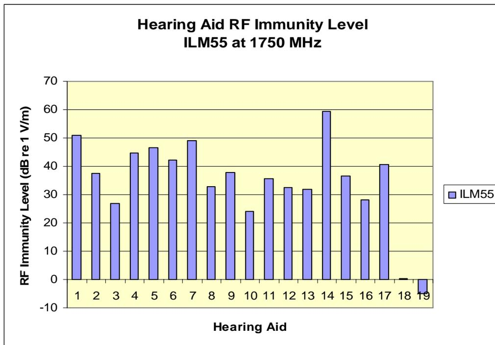
Figure 11: The radiofrequency immunity level for each hearing aid in microphone setting measured at 1750 MHz.
