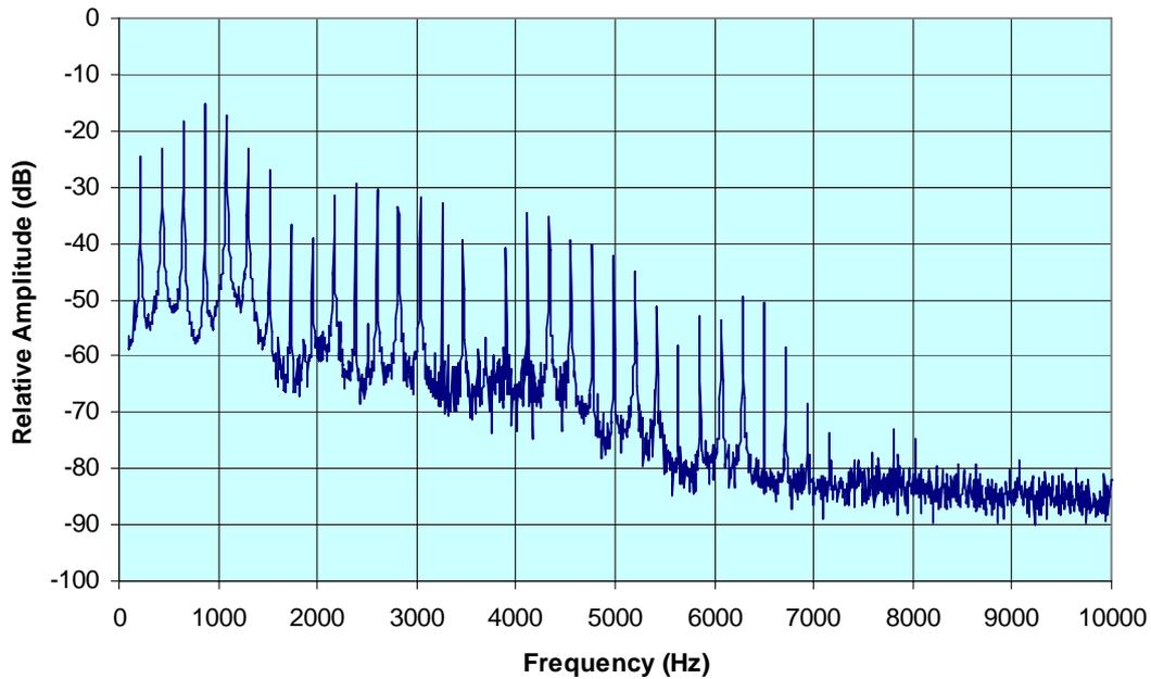
**Figure 7:** Spectral response of interference produced in a radiofrequency medium immunity hearing aid at reset volume control and placed next to a 1750MHz GSM Mobile transmitting on full power.
