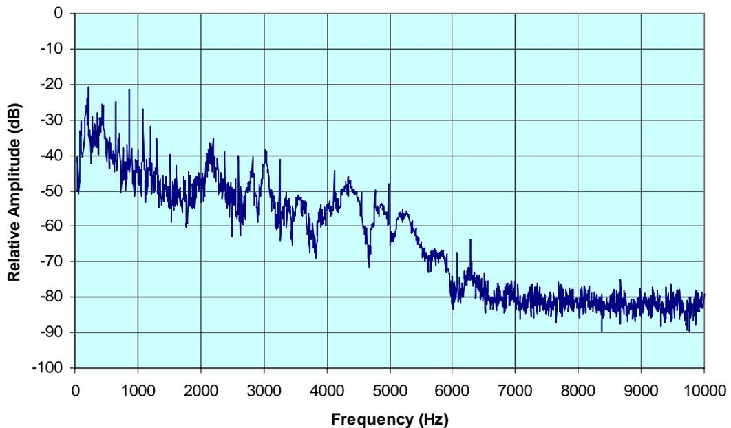
**Figure 9:** Spectral response of interference produced in a radiofrequency high immunity hearing aid at reset volume control and placed next to a 1750MHz GSM Mobile transmitting on full power.
