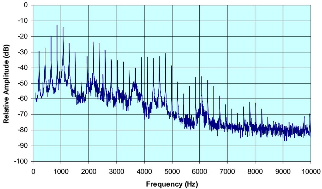
**Figure 6:** Spectral response of interference produced in a radiofrequency low immunity hearing aid at maximum volume control and placed next to a 1750MHz GSM Mobile transmitting on reduced power, -13.4 dB re maximum output (nominally -14 dB re maximum output).
