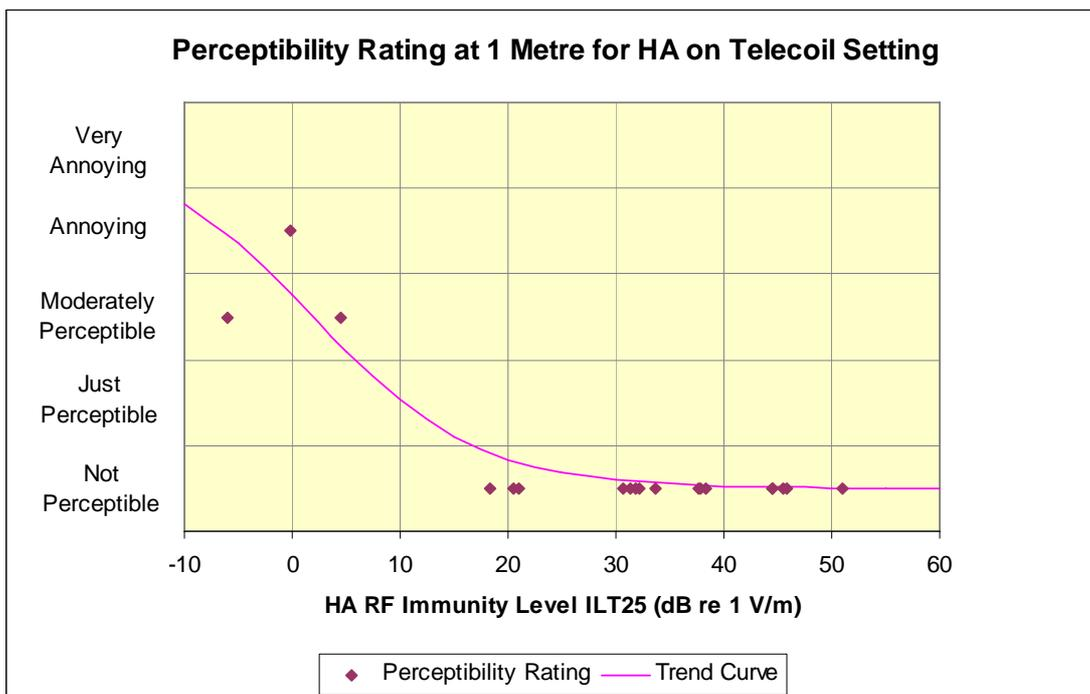
**Figure 14: The perceived interference with the hearing aids in telecoil setting and positioned 1 metre from the mobile transmitting at maximum power level.**
