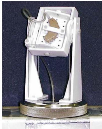
**Figure 3: Typical mounting of a BTE hearing aid in manipulator.**
