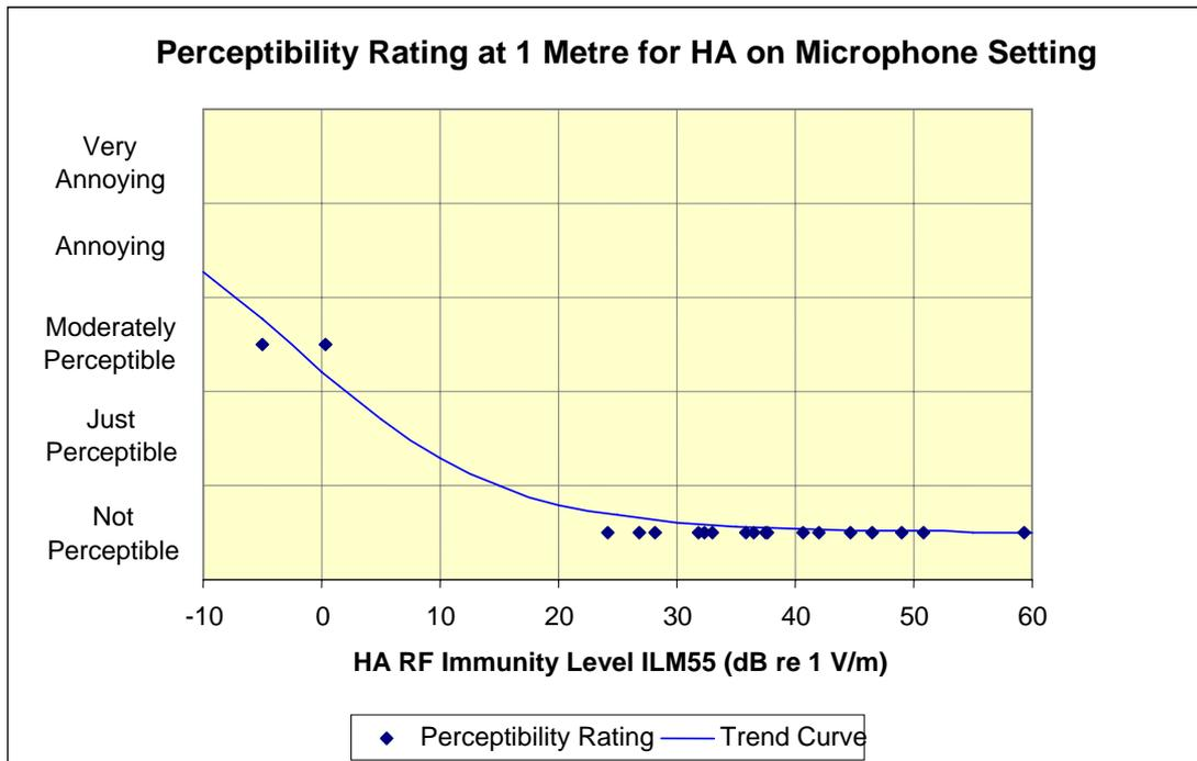
**Figure 13: The perceived interference with the hearing aids in microphone setting and positioned 1 metre from the mobile transmitting at maximum power level.**
