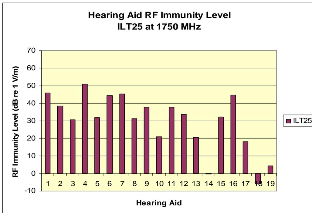
Figure 12: The radiofrequency immunity level for each hearing aid in telecoil setting measured at 1750 MHz.
