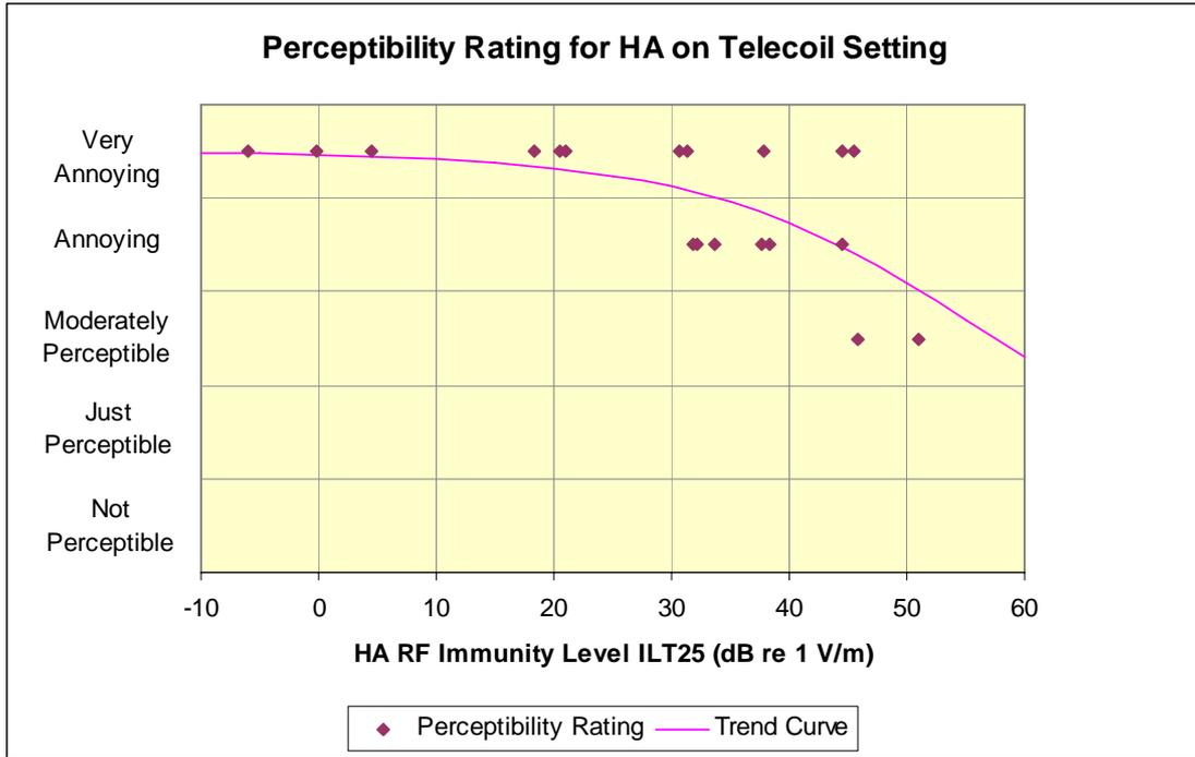
**Figure 19: Perceptibility rating of interference produced in hearing aids in telecoil setting by a 1750 MHz GSM mobile telephone operating at maximum transmit power level and held in normal listening position.**
