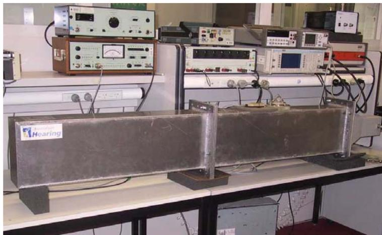
**Figure 1: Waveguide test apparatus set up for operation between 1700 and 2000 MHz.**
