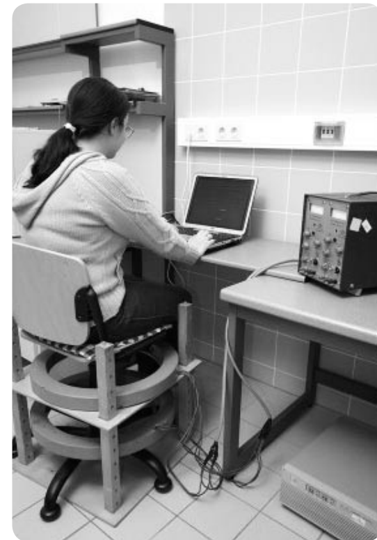
A subject sits in a chair above two large electromagnetic coils which are not connected to anything.
